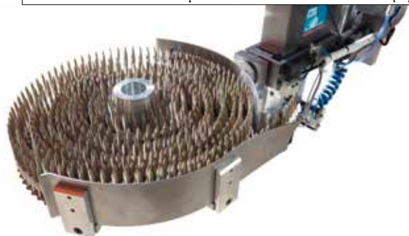
Jumbo coil: Magazine capacity 700 screws
